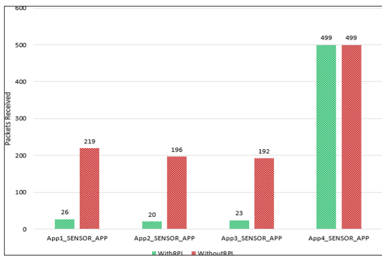
Figure 15. Packets received over the application sensor with and without RPL
